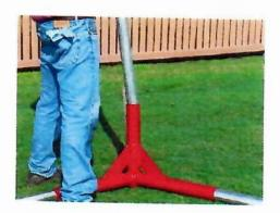
Insert the upright into the upright pipe on the stand with the slots lined up with the legs
