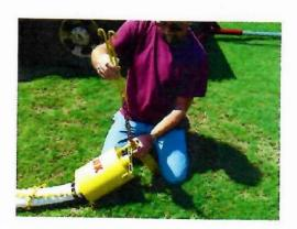
Place the chain onto the spring rod with the round end and feed the chain and rod through the spring from the tank end.
