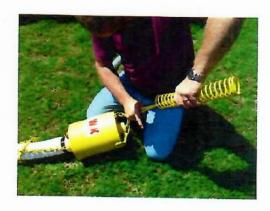
Pinch the end of the spring rod so that the hooked ends are beside one another and insert spring.
