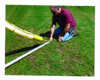
Pull the chain on the other end and hook it in the slot of the leg that is in line with the slot you used on the upright. It is best with 2 people, one person pulling down on the tank to compress the spring and the other person hooking the chain in place. If installing more than one scratcher repeat steps. If installing the scratcher on the supreme or ultimate the process is the same.
