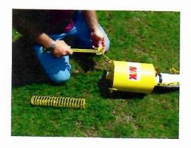
Run the spring rod with the square end through the chains on the top of the tank until the chain is in the corners of the square end.
