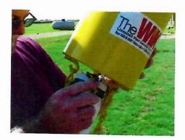
Hook the chains onto the tabs on the bottom of the tank. Make sure the flanges on the wik roll cap are placed over the tabs.
