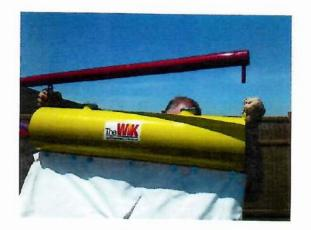
With the hooks provided hook the dairymatic to the loops on the support bar.
